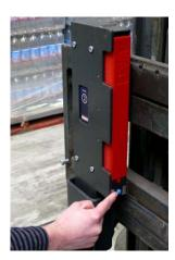
The indicator also uses an auto-shut-off mode: this one is standard activated after two minutes of not using the indicator keys. Fifteen seconds before switch-off a countdown routine starts in the display. By pressing any key during this countdown, the auto-shut-off function is interrupted and a new two minute cycle starts. From the auto-shut-off mode the weighing system is activated via the normal on/off key: within seconds the Bluetooth connection with the forks is restored.
