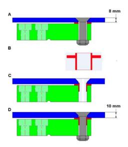
An extra 2mm of material has been added to the fork shoe: the thickness of the shoe is now 10mm instead of 8mm. This will prevent bending, even with longer forks and under maximum load. The washer between load cell and fork shoe (see drawing A) has been replaced by a cylindrical bush (B-D). The bush absorbs horizontal forces and prevents loosening of the bolts.
